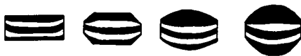
FIG. 2. Compacts showing axial powder movement prepared using an axial compressive force of 98.1kN.
